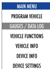
3. On **initial setup**, you will need to select **Configuration** press the **center button**, and **select your vehicle** from a list of data log files. In the future, you can continue without going through the vehicle selection.
