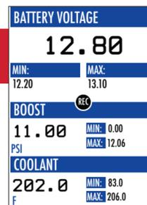
5. The items being monitored can be adjusted by pressing up or down on the device to highlight and then pressing the center button on the BDX to select which reading you'd like to change. Within this menu, you can change the item you're monitoring, and the units in which it will be displaying. You can also change the layout of the gauges within this menu.
